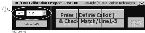
Figure A-5 Performing 2-port TRL/LRM calibration
